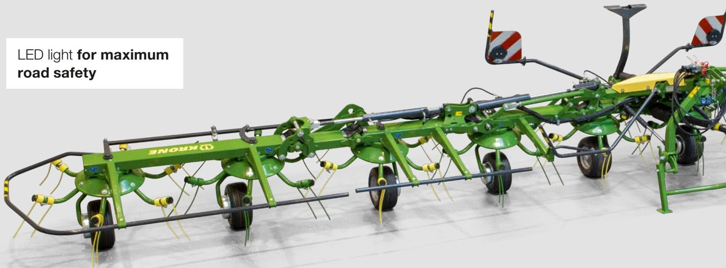
Gauge wheels run close to the tines providing **exact tine control and optimum forage quality**
