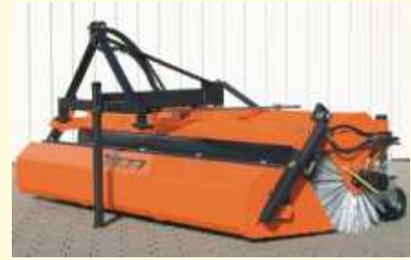
bema 25 tractor mounting attachment with 3 point rear mounting (hydraulic waste collection container)
