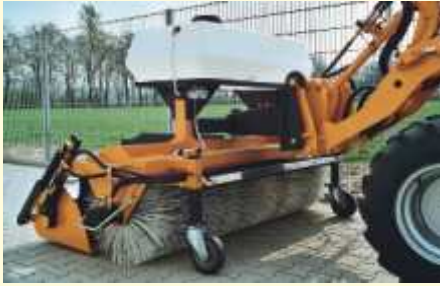
bema 25 complete (with quick change to wheel loader, water spray system 240 ltr., hydraulic side brush). Only one reversible hydraulic service is necessary for all functions.
