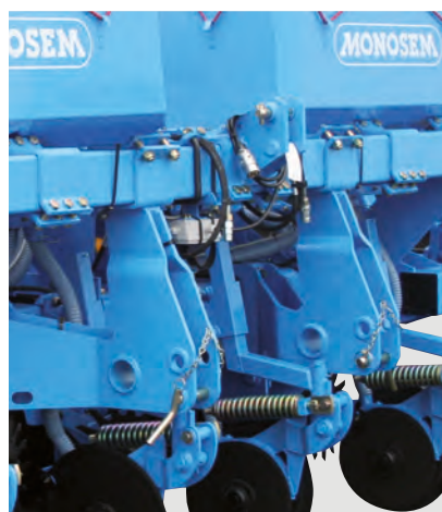
Hitch on rigid double bar frame
