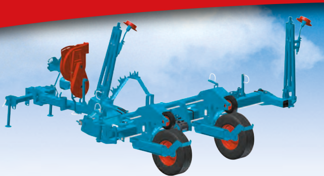
8-row WingFold pull-type planter with fertilizer (inter row 75 cm)
