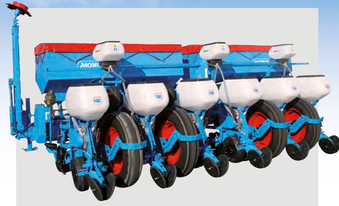
6-row pull-type planter with fertilizer (inter row spacings of 75cm)
