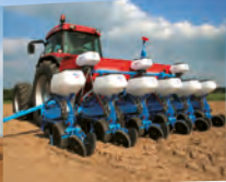
Multi-purpose pneumatic NG Plus 4 planter with discs
