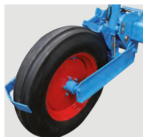
Wheel unit on pull-type frame with 7,5 x 20 wheel. (235 x 75 wheel on 6 and 8-row WingFold)
