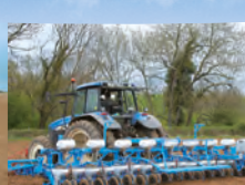
Mechanical planter for pelleted sugarbeet MECA V4
