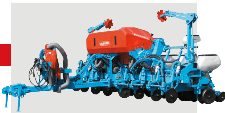
Fertilizer 1500 litres on 8-row folding pull-type WingFold planter
