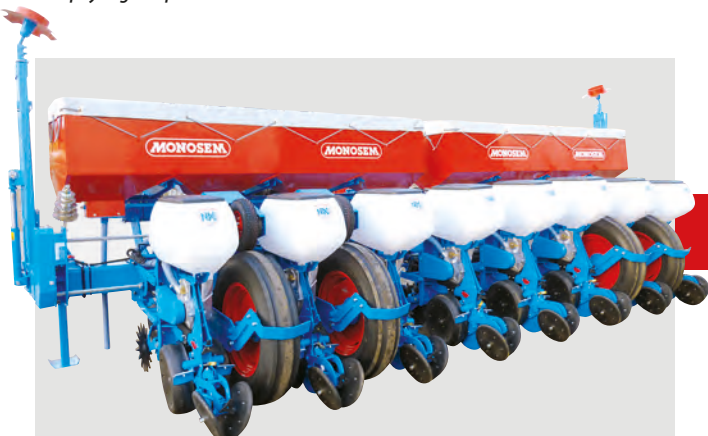
Fertilizer 2 x 1000 litres on 8-row rigid pull-type planter
