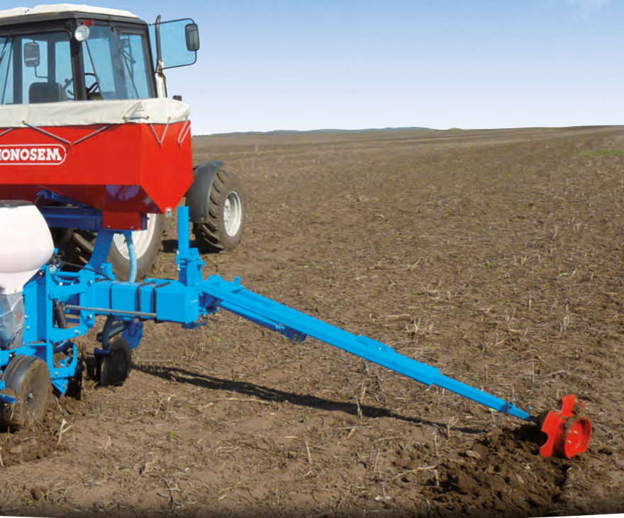
6-row pull-type planter with fertilizer (inter row spacings of 75cm)
