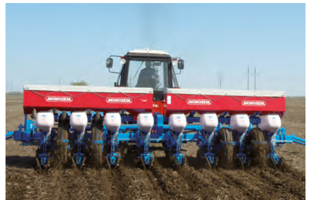
8-row pull-type planter with fertilizer (inter row spacings of 70cm)
