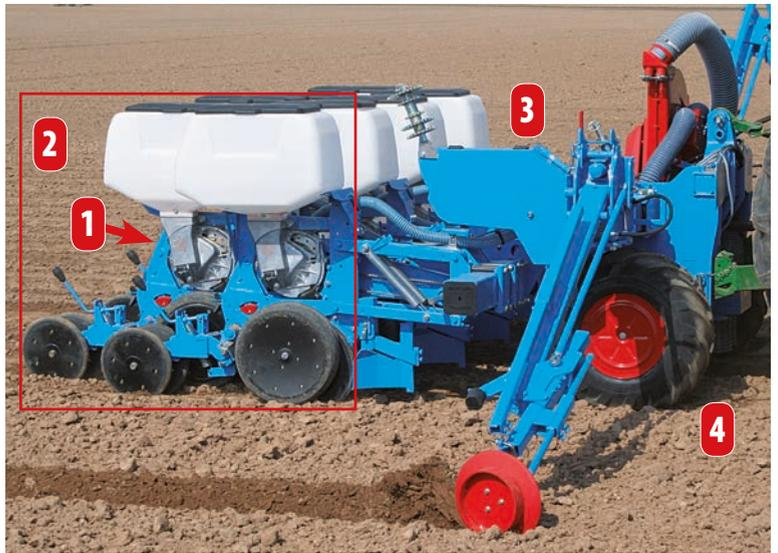
**4** The Twin-Row planters are equipped with front wheel units for clearance between the metering units.
