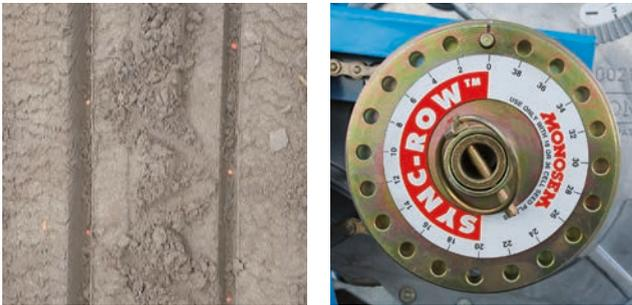
**2** The planting of each double line is ensured by 2 independent metering units for optimal planting.
