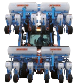
The central part of the frame is made up of a double telescopic frame, the wings are telescopic and folding for a transport width of 3m (depending on the equipment).
