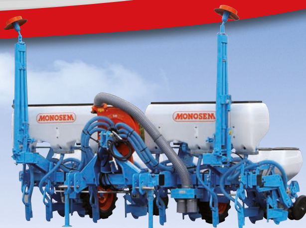
NC Technic Maize planter 6-row Monoblock Telescopic Frame Fertilizer 2 X 270L with knives
