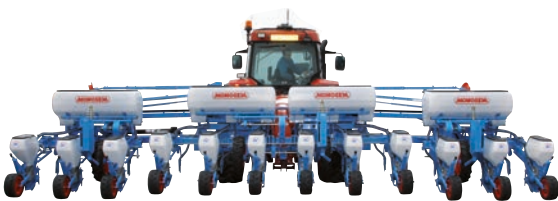
The central part of the frame is made up of a double telescopic frame, the wings are telescopic and folding for a transport width of 3m (depending on the equipment).
