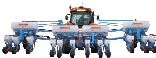
The central part of the frame is made up of a double telescopic frame, the wings are telescopic and folding for a transport width of 3m (depending on the equipment).
