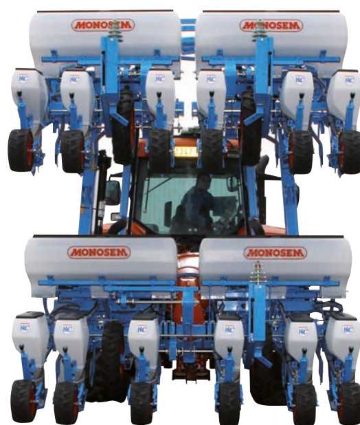
* Example of CRT frame folded at 3m00
