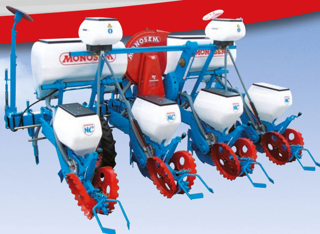
NC Classic V1 planter 4-row Monobar rigid frame (75 cm) Microsem and Fertilizer 2x175 L with knives
