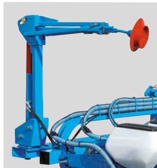
The row markers on double bar folding frame and CRT frame enable a compact folding for a minimum transport dimension.
