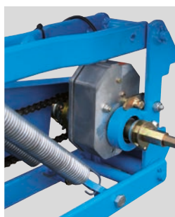
Electromagnetic clutch on NC metering unit
