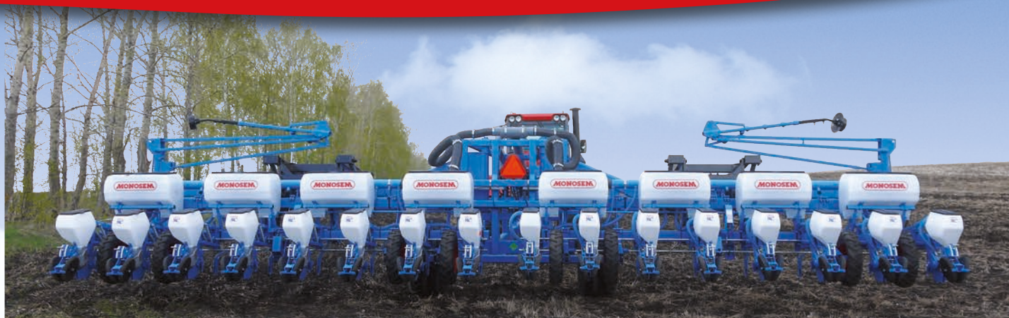
NC Technic Maize planter - 16 rows at 70 cm Combining 2 rigid double bar 8-row frames with fertilizers 4 x 175L with knives on toolbar
