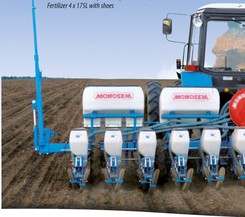
12-row NC Technic Sugarbeet rigid monobar planter (45 cm) Fertilizer 4 x 175L with shoes
