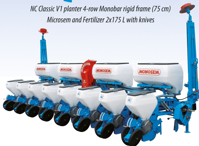
NC Technic Maize planter 8-row Monobar rigid frame (70 cm) Fertilizer 4x175 L with knives
