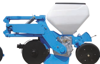
NC Technic Maize metering unit Rear gauge Double-discs
