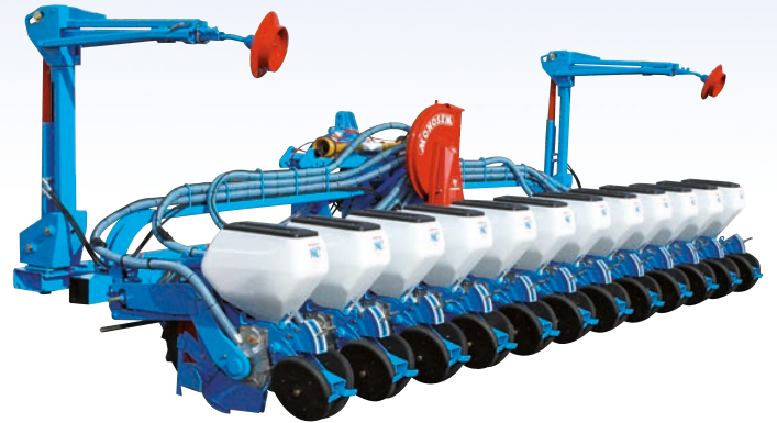
NC Technic Maize planter 12-row double bar folding frame (45 cm)
