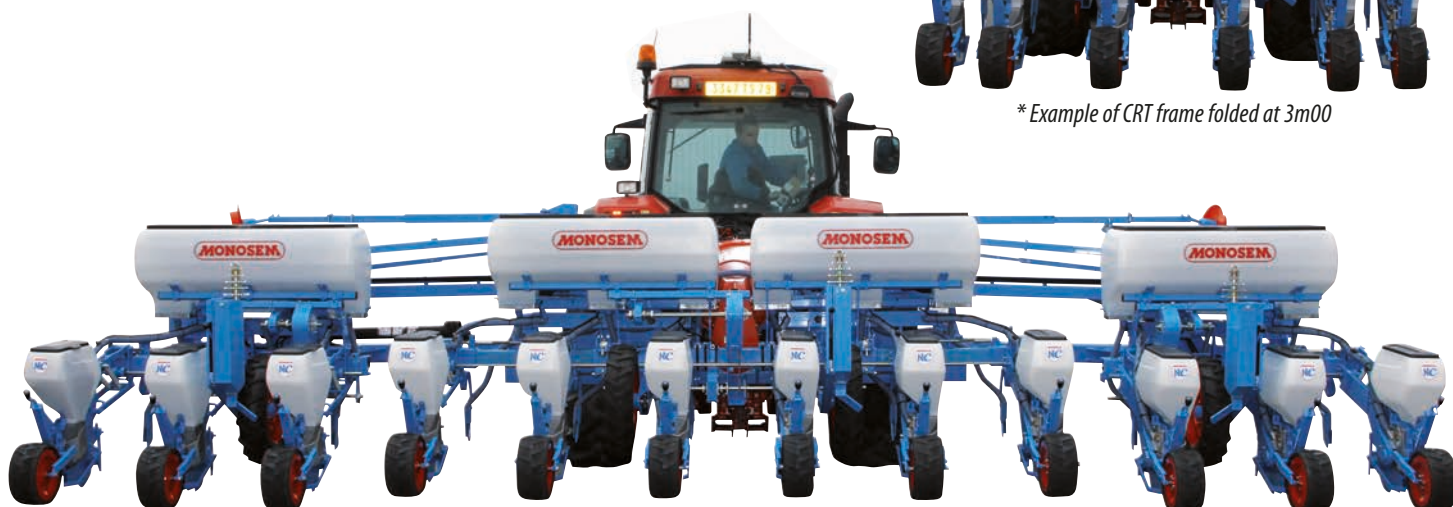
NC Classic V2 planter - 12 rows at 75 cm Folding CRT frame - folds to 3m00 *
