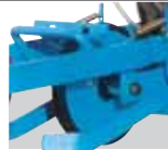
Intermediate press wheel with self-cleaning supple tyre
