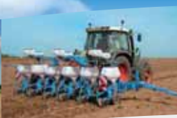
Special pneumatic « low-till » planter NX 2 with discs
