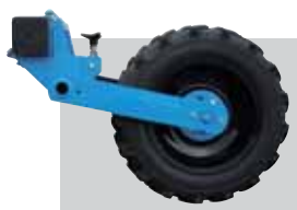
Adjustable wheel unit with 6,5 x 80 x 15 wheel Minimum inter-row spacings (1) : 45 cm Wheel clearance: 19 cm
