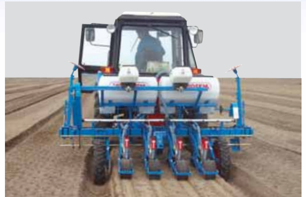
MS A Planter - Monoblock rigid frame - 4 rows with fertilizer and Microsem
