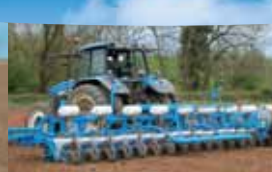
Mechanical MECA V4 planter for pelleted sugarbeet
