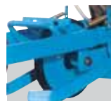
Intermediate press wheel with self-cleaning supplie tyre
