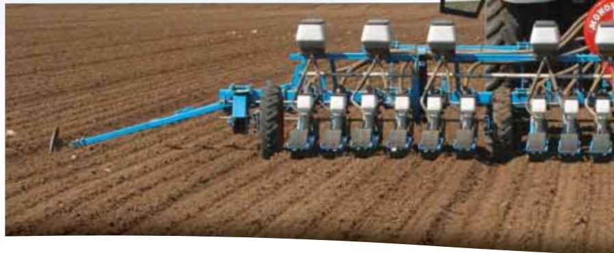
MS A Planter - Double bar rigid frame - 3 x 6 rows with Microsem
