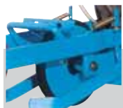
Intermediate press wheel with self-cleaning supple tyre (not compatible with the MS D metering unit)
