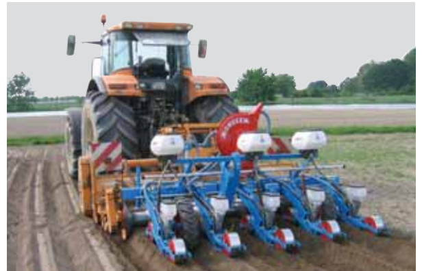
MS A Planter - Monobar rigid frame - 5 rows with Microsem
