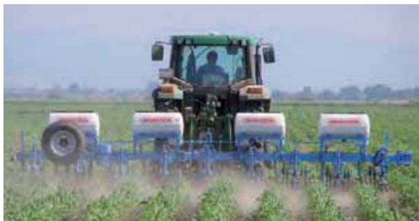
TIP 5" rigid SCD cultivator - 8 rows at 70 cm inter row spacing at work
