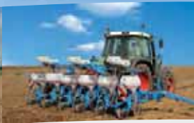
Special pneumatic « low-till » planter NX 2 with discs
