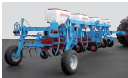
TIP 5" rigid SCD cultivator - 8 rows at 70cm inter row spacing in transport
