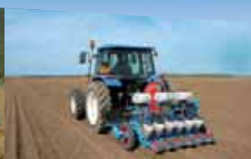
Mechanical MECA V4 planter for pelleted sugarbeet
