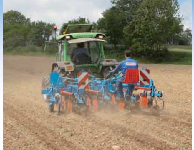
The steering wheels (1), orientated by the steering bar (2), can be adjusted in height (3).
