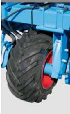
The wide wheels with large diameter ensure a regular and constant drive of the seed discs. The rapid adjustment of the width of the drive wheels means a rapid adjustment to the different tractor treads.
