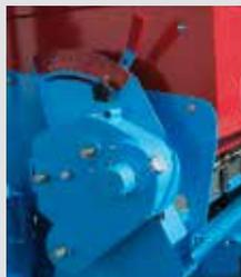
Easily accessible on the side of the planter, the FertiDrive<sup>VM</sup> variable speed transmission allows very quick and easy adjusting of the quantity of fertilizer per hectare required. This transmission is also equipped with a disengaging mechanism, used to stop the fertiliser intake where it is not necessary.
