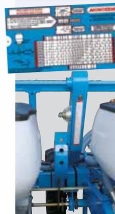
Adjustment of the microgranulators is made using a gearbox with 18 ratios. If needed, other sprockets are available and also a rapid declutching system. The adjustment chart delivered with the Microsem enables a rapid adjustment of the quantity of product.
