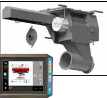
On the Standard and DUO front-mounted hoppers with electric drive, the quantity of fertilizer is managed from the tractor cab via the ECU F800E and the ISOBUS touch terminal (TOUCH or TOUCH Mini). The front fertilizers with electric drive have an easily-removed and without tools dosing wheel and metering anticipation function.
