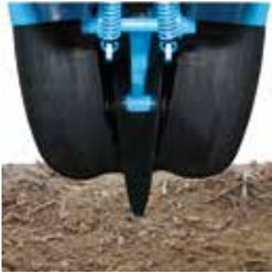
*The double discs open the furrow at a depth defined by the gauge wheels.*
