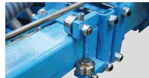
The roller bearings mounted on bushes enable a perfect operation of the double telescopic frame year after year.
