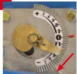
*For the large seeds, suction is maximum and the selector is adjusted according to the size of the seed.*
