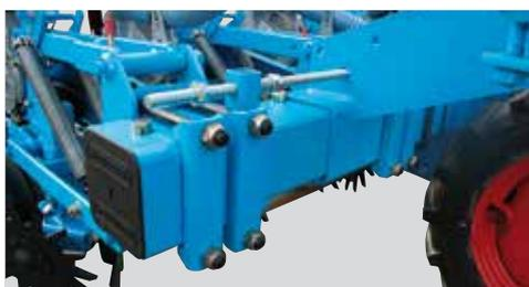
The stop parts on the telescoping system enable an adjustment perfectly suited to the required inter row spacing and folding that is suited to the equipment of the planter.
