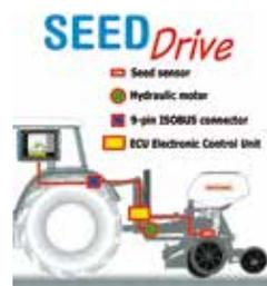
The SeedDrive hydraulic control of the seed population replaces the planter seed spacing gearbox(es) by several hydraulic motors which drive the seed discs. This system offers the possibility of non-stop modulating of the seed population directly from the tractor cab with the TOUCH Mini or TOUCH terminal or another ISOBUS compatible terminal.
