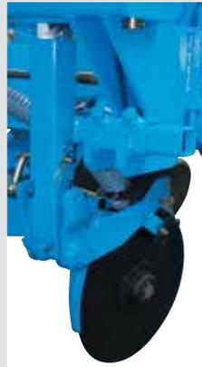
On the Extend planter, a Double function turbofan (Df) ensures an efficient vacuum suction of the seeds and also to pulse the fertilizer on the outer rows to efficiently distribute at 45 or at 80 cm inter row spacings. On the pulsed rows, a stainless steel cyclone is integrated on each fertilizer disc.
