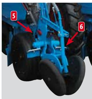
The Insecticide Microsem chute (5) is placed between the 2 discs for product supply in the planting line. The Helicide Microsem chute (6) is adjustable for a product supply on the planting line before or after the passage of the press wheels.
