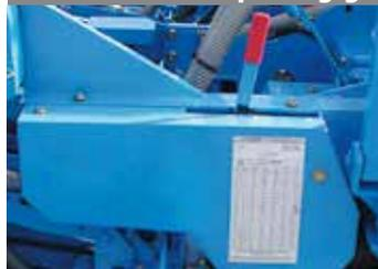
The drive of the metering unit is ensured by a reinforced transmission. The seed spacing gearbox is situated on the extreme left side of the planter for easy access and a rapid changing of the sprockets. The 20 settings with interchangeable sprockets offer a wide choice of seed populations.
