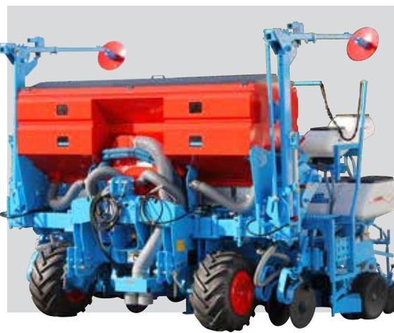
The « High Capacity » hoppers in sheet metal on the single and double telescopic Monoblock2 Comfort frames have a capacity of 680 L or 1030 L. On the Extend frames, the capacity is 1020 L. This capacity is 1500 L on the TFC folding frames.
