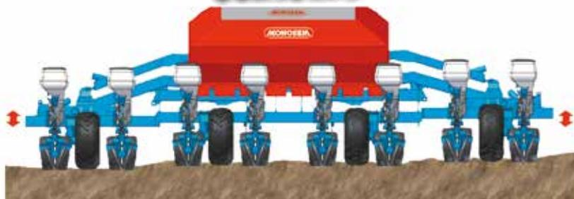
The floating Double bar folding and the floating TFC frames have independent wings with wheel units. This characteristic allows for a perfect following of the ground. At the field ends or to finish off a field, it is also possible to lift one or other of the wings (or the 2) thus automatically stopping the metering.
