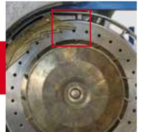
*For the small seeds, the suction is reduced simultaneously to the selector adjustment.*
