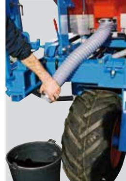
The « High Capacity » fertilizer hoppers are equipped with a trapdoor on each side with a hose enabling a rapid and easy emptying of the hoppers.
