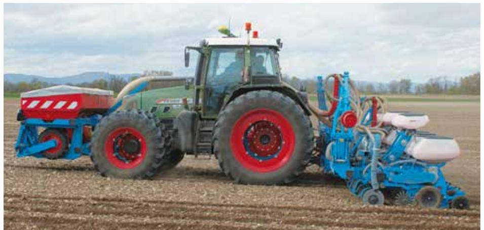
The CRT frame can be equipped with standard fertilizers (4 x 270 L) or the equipment for the front-mounted Standard or DUO fertilizer. In this configuration, the planter has 2 distribution heads (assembly according to inter row and equipment).
