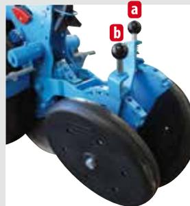
The Monoshox NG Plus M unit is equipped with a rear press wheel unit that can be adjusted using levers\*.
