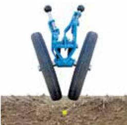
*The adjustable open press wheel unit\*, made up of 2 V-wheels, closes the furrow around the seed for optimal seed germination.*
