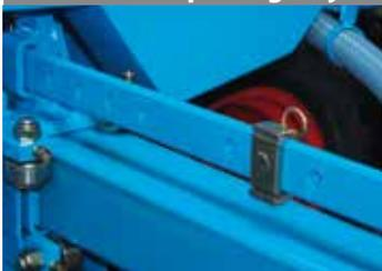
The adjustment of the inter row of the Extend planter is very simple. You just have to position the stop parts on the adjustment bar on the required spacings and then lengthen or shorten the hydraulic cylinders on the telescopic bars in order to obtain the desired spacing.
