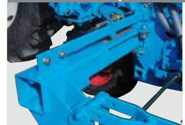
The hydraulic telescopic bars ensure the lateral movement of the metering units in order to change inter row spacings. In order to limit friction and ensure a longer life, the bars are equipped with guiding bearings mounted on bushings.
