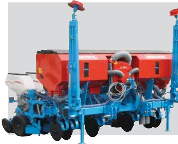
The « High capacity » hoppers in sheet metal on Monoblock, single or double telescopic frames have a capacity of 980 L.
