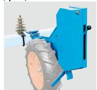
For even easier access, a rear seed spacing gearbox with integrated wheel unit is also available. This seed spacing gearbox with interchangeable sprockets gives and even more precise adjustment for seed population.
