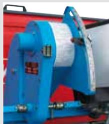
The Microsem has a MicroDrive<sup>VM</sup> variable speed drive easily accessible for a quick and easy adjusting of the required dose. This transmission is also equipped with a disengaging mechanism, used to stop the Microsem intake where it is not necessary.
