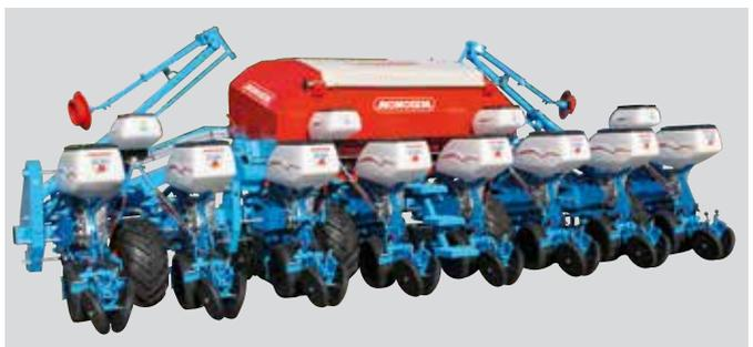
8-row TFC floating frame (75 cm inter row spacing) with fertilizer and Microsem
