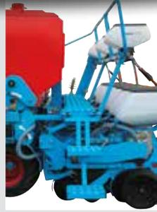
On the Extend planters with fertilizers, a platform, delivered as standard equipment, enables an easy access to the fertilizer hopper. The platform and the step thus enable a safe access to the hopper during filling operations.
