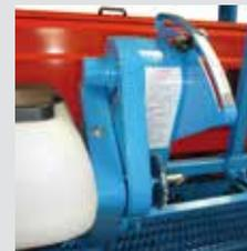
The Microsem has a MicroDrive<sup>VM</sup> variable speed drive easily accessible on the side of the planter for a quick and easy adjusting of the required dose. This transmission is also equipped with a disengaging mechanism, used to stop the Microsem intake where it is not necessary.
