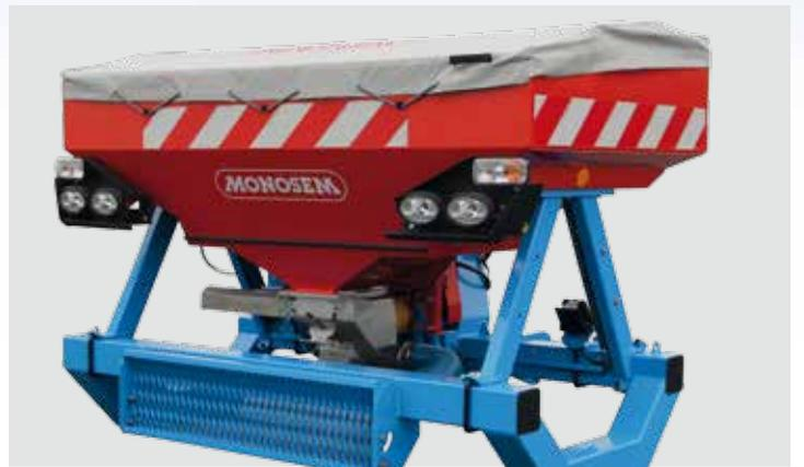
The standard front hopper is available with capacities of 1000L or 1600L. The unit can be assembled on planters up to 12 rows. This fertilizer has a stainless steel metering system and an electric drive for a rapid adjustment of the quantity of fertilizer to be distributed.
