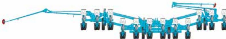
The central part of the frame is made up of a double telescopic frame, the wings are telescopic and folding for a transport width of 3m (depending on the equipment).
