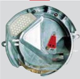
The cover in alloy is specially designed for planting with a minimum of seeds.
