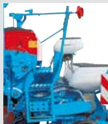
On the Monoblock2 Comfort planters with fertilizers, a platform, delivered as standard equipment, enables an easy access to the fertilizer hopper. The platform and the step thus enable a safe access to the hopper during filling operations.
