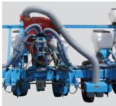
According to current law, MONOSEM can propose anti drift of dust kits (KAP). These kits are approved by the BBA Germany and guarantee the correct operating of MONOSEM planters.
