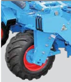
The wide wheels with large diameter ensure a regular and constant drive of the seed discs. The rapid adjustment of the width and the height means a rapid adjustment to the different planting conditions.
