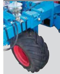
The wide wheels with large diameter ensure a regular and constant drive of the seed discs. The rapid adjustment of the width of the drive wheels means a rapid adjustment to the different tractor treads.
