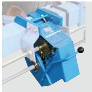
The standard seed spacing gearbox with 18 ratios gives a rapid and precise adjustment of the seed population. Changing the seed population is rapid. A single lever releases the chain. Then just place the required sprockets facing each other and release the lever to re-tighten the chain.
