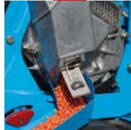
The emptying trapdoor offers optimal operating. Open the trapdoor and it stays open enabling, with the emptying auger supplied as standard equipment, an even easier and more efficient emptying.
