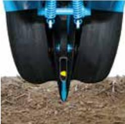
*The V-tip finishes the bottom of the furrow for an optimal seed placement.*
