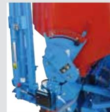
Easily accessible on the side of the planter, the FertiDrive<sup>VM</sup> variable speed transmission allows very quick and easy adjusting of the quantity of fertilizer per hectare required. This transmission is also equipped with a disengaging mechanism, used to stop the fertiliser intake where it is not necessary.
