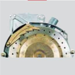
The brass scraper avoids doubles. A spring on the metering box cover maintains the selector perfectly in place against the disc for optimal selection, even with small seeds.
