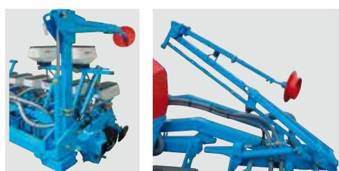
The row markers on double bar folding frame and TFC folding frame enable a compact folding for a minimum transport dimension.
