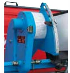
Available on option on certain models, the MicroDrive™ offers a rapid and precise adjustment of the dose to be applied.
