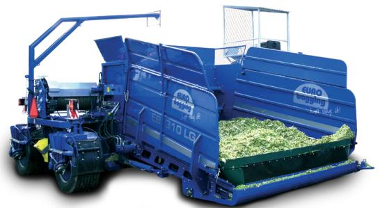
The most popular silage bagging machine of its type for storage of grass haylage, maize silage, sugar beet pulps, by-products, CCM or brewer's grain. The unique QUICK system allows quick preparation of the machine for operation. Comfortable hydraulic accessories with proportional control of the main control functions.
