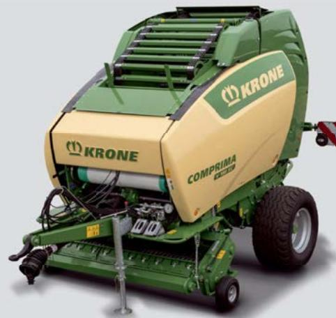
set to handle all crops and conditions. Smaller bale sizes are often preferred in grass silage whereas larger bales are more typical in hay and straw. It is also possible to choose a softer core, which is useful in hay, for example, as it allows moisture to evaporate from the bale.
